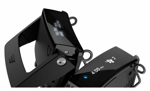
The Reflex device is about the size of a deck of cards and attaches to your belt or waistline. Once clipped on, its sensors measure how the body moves, determining if an unsafe movement, or high risk posture (HRP) has occurred.
