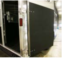
New composite rubber wall lining in horse area
