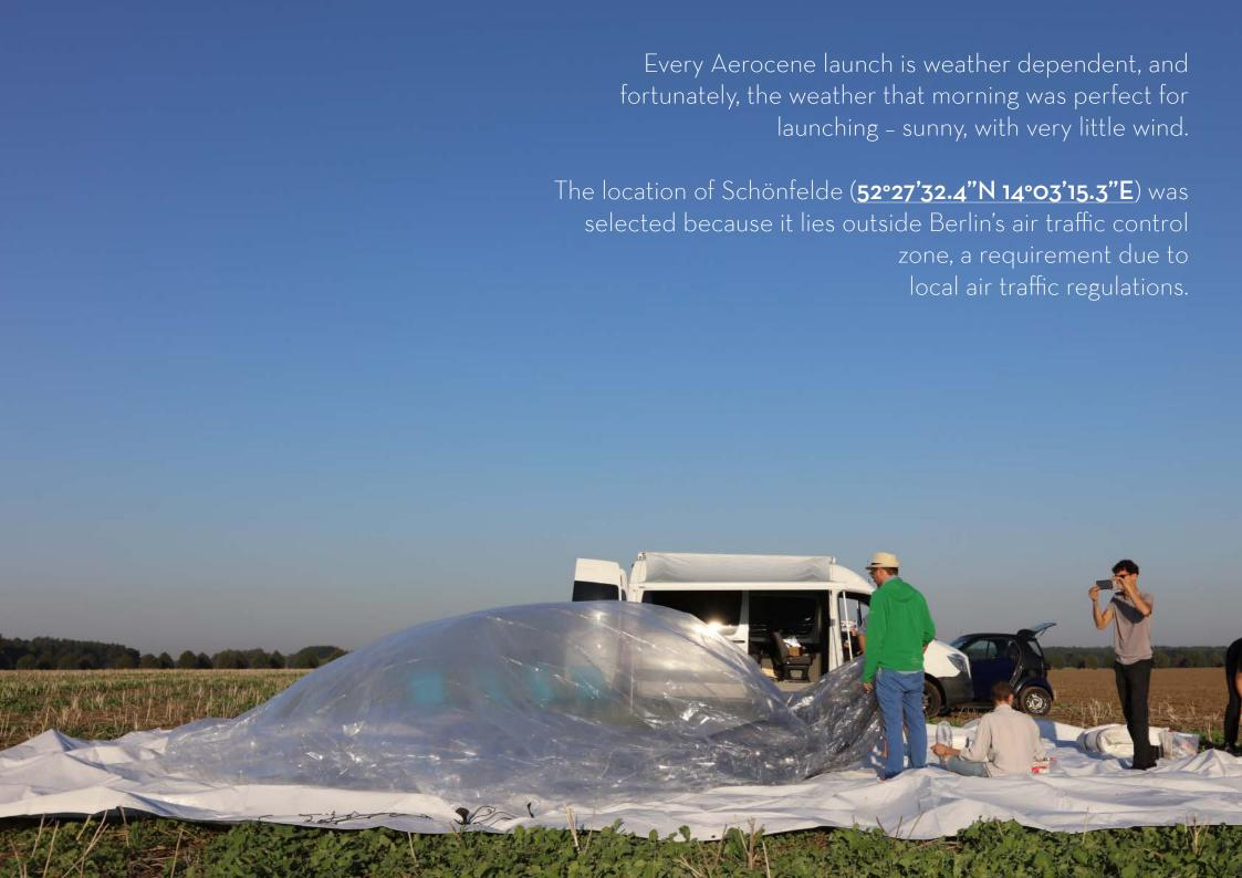
We spread white tarps on the ground to increase the **albedo** of our launching surface. Launching from a light-colored surface reflects the intensity of the sun's rays on the sculptures, resulting in greater buoyancy.
