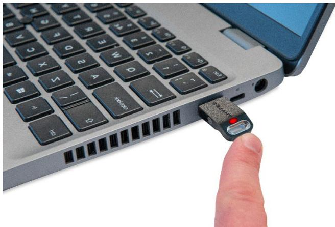
On a PC, tap the security key while it is inserted to complete authentication.
