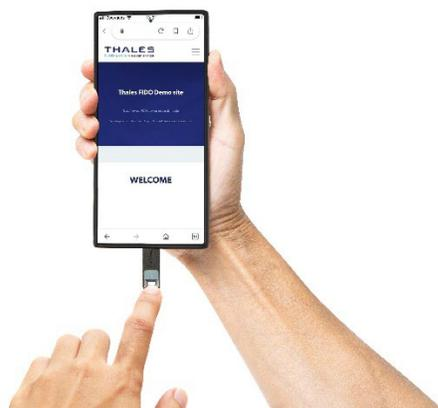
On a mobile device, tap the security key while it is connected to complete authentication.
