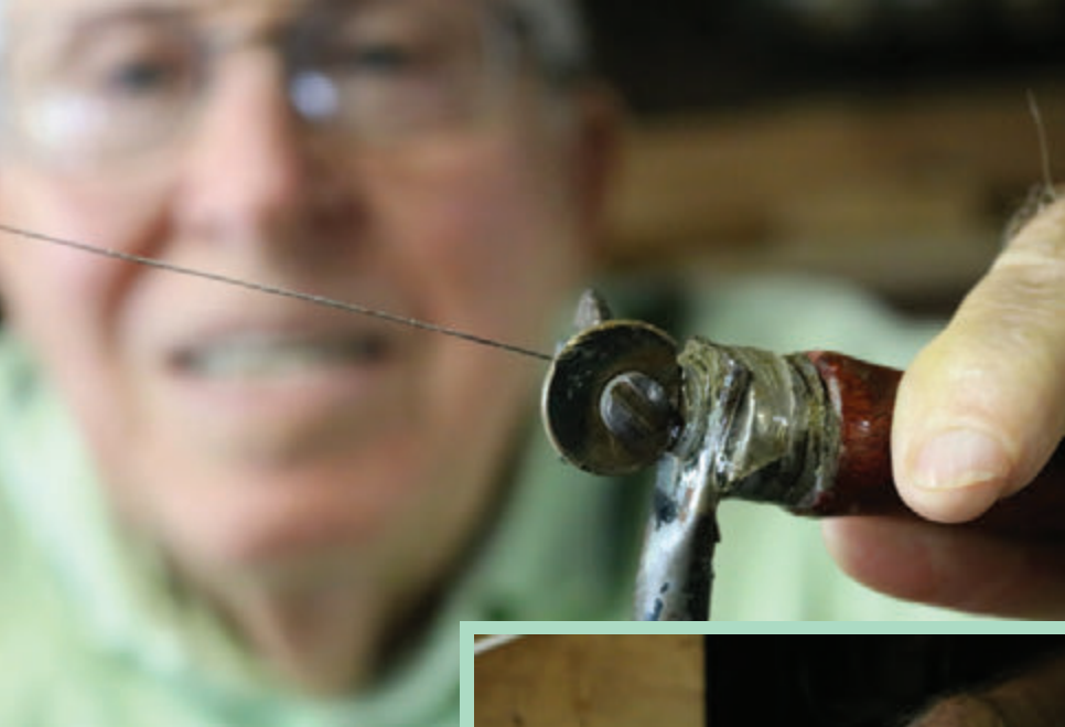
Del Porter repairs his broken saw blade while working on a marquetry project. The blade of the saw is as thin as a horse hair, and needs to be threaded very carefully to prevent it from breaking.
