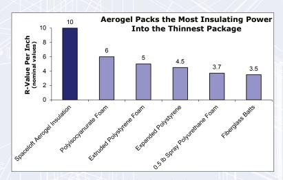
$\ensuremath{\mathsf{R}}$  means resistance to heat flow. The higher the R-value, the greater the insulating power.
