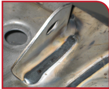
Clean Lincoln production weld on mild steel chassis part
