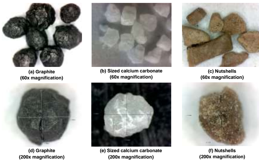
Fig.8 Optical microscopy images of the three LCMs
