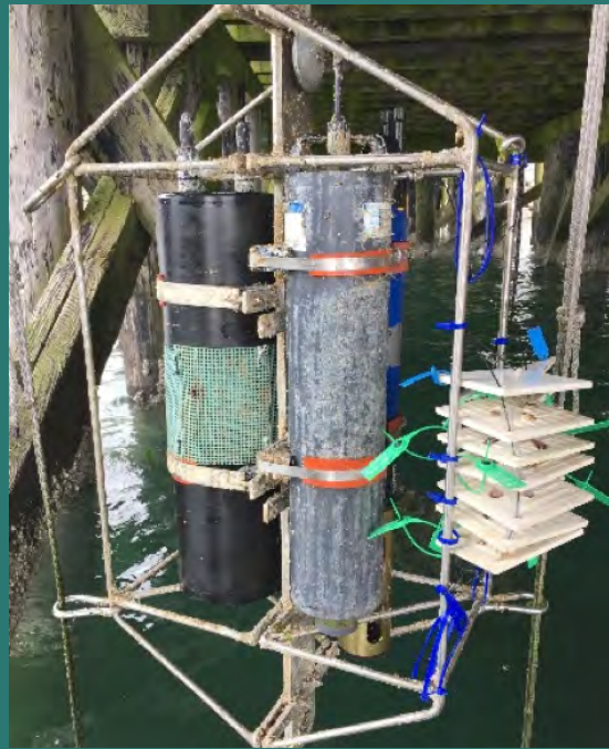
Sensors measure acidity and CO 2 , dissolved oxygen, chlorophyll a, temperature, salinity, and water depth.
