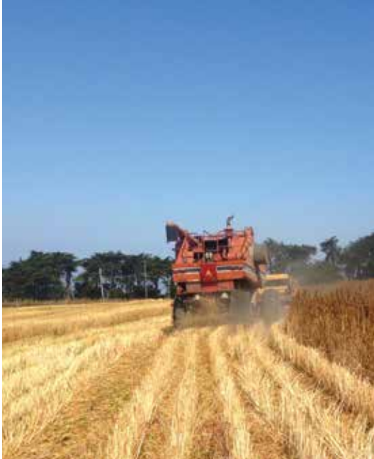
A combine harvests Cherry Vanilla quinoa near Elk, California. The combine cuts the dry stalks and separates the seed from the straw through an onboard threshing process. The machine then sifts the grain from other organic matter. Lundberg is careful not to discard the excess, because some of the tiny seeds don't make it into the combine's grain bin.
