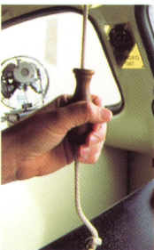
One sentimental holdover remains from the locomotives of old: a whistle cord.
