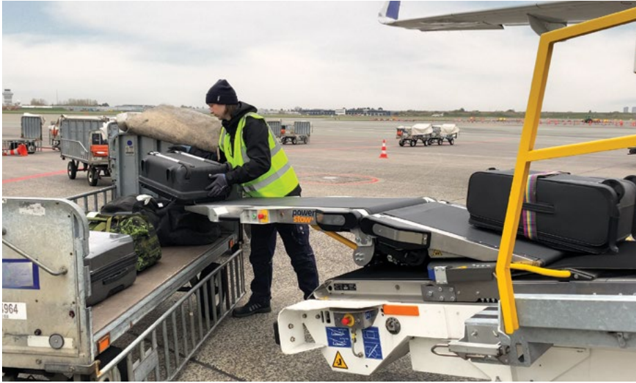
Power Stow launched the Tail Loader at the end of last year as an ergonomic lifting device aimed at bridging the gap between the belt loader and a baggage cart. Image: Power Stow
