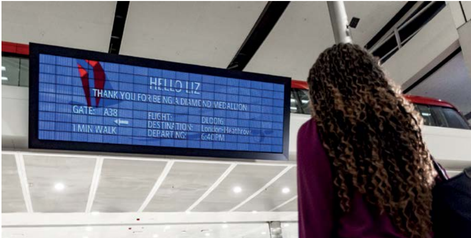
Similar to a technology predicted in the 2002 film Minority Report , Parallel Reality displays uses multi-view pixels that can project individualised content to people viewing the screen.
