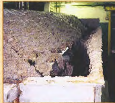
The clean pulp enters a thickener before it proceeds to a paper machine.
