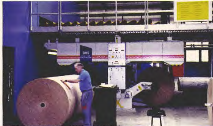
Model's new BHS corrugator replaced two older corrugators.
