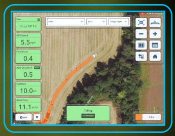
The FieldView Drive is an equipmentagnostic device that reads operationally relevant messages from a CAN diagnostic port and transfers them to the FieldView Cab app via Bluetooth®, enabling real time in-cab data visualization and insights, as well as farmer options for data sharing
