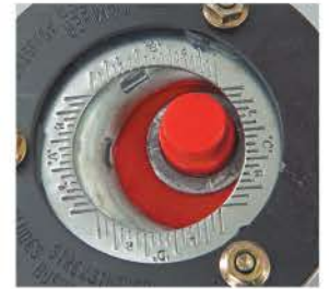
Front camber kits have indicators to help you mark your settings so you can quickly and accurately change from street to track, and back.
