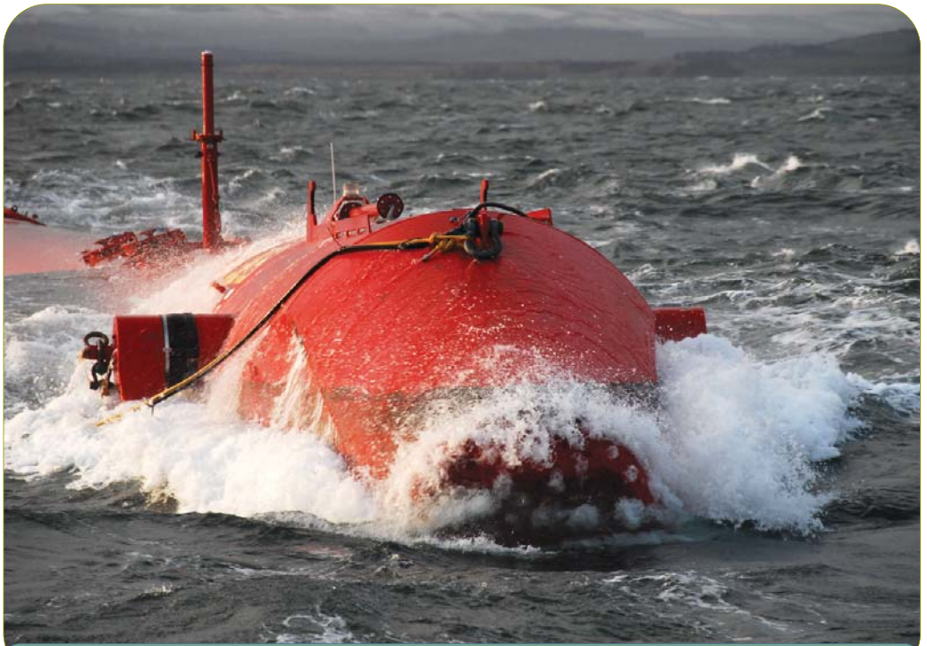
The Pelamis turns uses a hydraulic system to turn wave motion into energy. PHOTO: John Paul Photography
