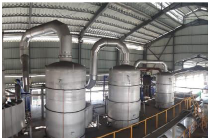
Alfa Laval POMEvap is compact, versatile and has a small footprint compared to the conventional ponding system
