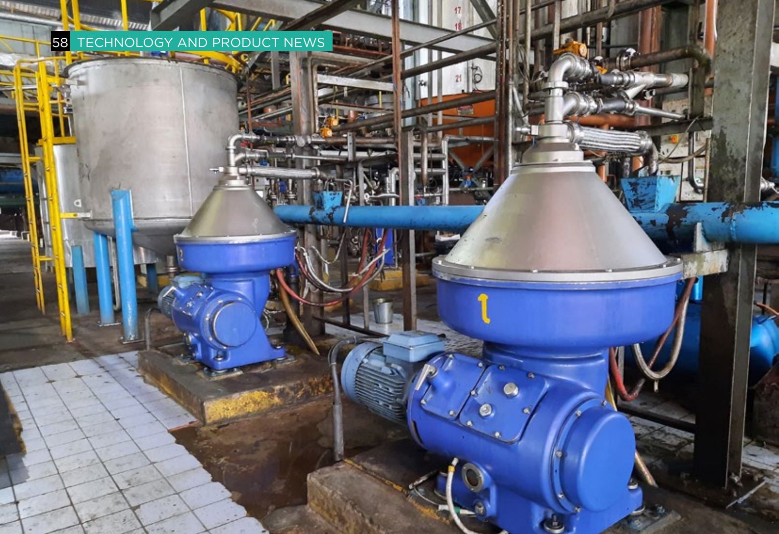
Alfa Laval's separators: Two units of VO30 at Leepang Palm Oil Mill
