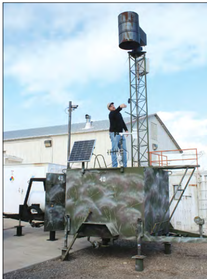
MODIFYING THE MODIFIERS: Jesse Juchtzer of the DRI works on one a cloud seeding generator outside the DRI’s manufacturing shop in Stead, Nev. Photo by Dave Zook/Moonshine Ink
