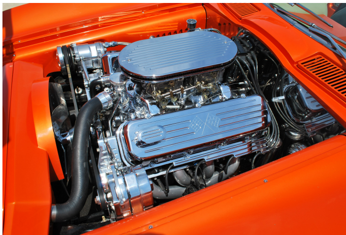
A polished 1970 LS6 454 big-block anchors the show-ready engine bay, backed by custom wiring and a three-inch exhaust.
