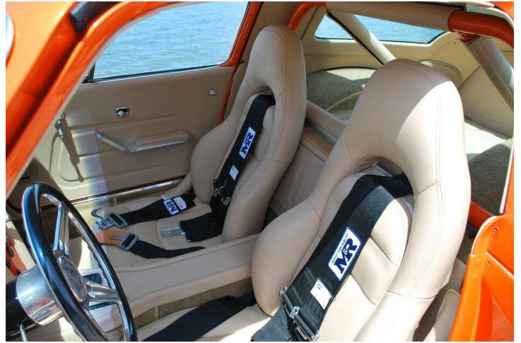
The custom cabin combines 1997 Corvette sport seats, racing harnesses, a leather-wrapped roll bar and a one-off console.
