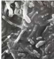
Biofilm found in water lines
