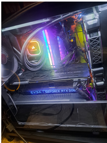
Internal packaging and clearance: full-performance desktop hardware integrated within the limited volume of the Mini-ITX enclosure.
