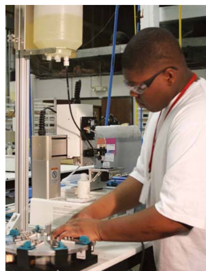
Left: Recycling more than one million empty cartridges every month. Right: Testing ultrasonic welding versus adhesive attachment of caps to cartridge bodies.
