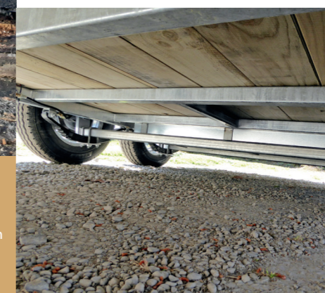
LEFT An angle loader can offer a more inviting space for green or nervous travellers when loading. ABOVE Moisture had rotted the untreated plywood floor in this float. RIGHT If you're buying second-hand, check the floor from underneath.
