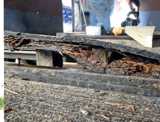
LEFT An angle loader can offer a more inviting space for green or nervous travellers when loading. ABOVE Moisture had rotted the untreated plywood floor in this float. RIGHT If you're buying second-hand, check the floor from underneath.
