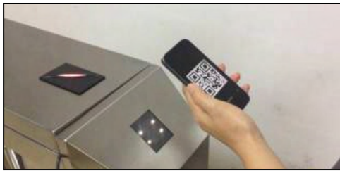
Fig: Self-Scanning Turnstile that is able to scan any QR Code regardless of third-party provider. Admission will be allowed as long as they have the correct ticket for the attraction entered.
