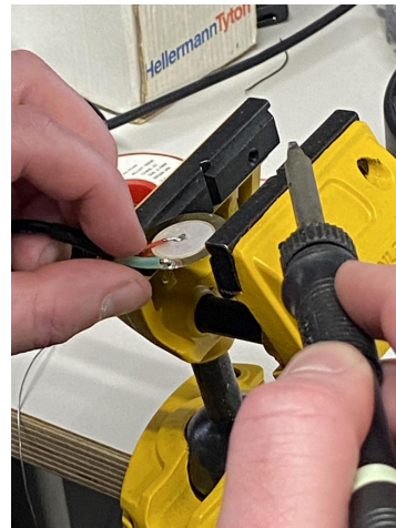
Figure d. The other end of the XLR cable is cut to reveal the conductor wires (not pictured). The red, or positive conductor wire, is soldered onto the positive ceramic plate close to center. The grounding and blue cable are twined together into a green insulation sheath and soldered to the outer ridge (negative).
