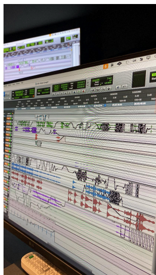
Figure g. Automation in touch mode in Pro Tools; this figure shows to which speaker and when each sound in each track is moving.
