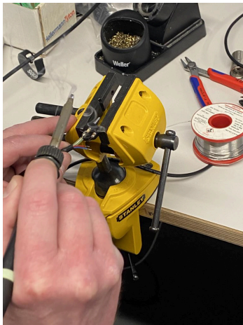
Figure c. The three conductor wires (already tinned with solder) are connected into the connector cups.
