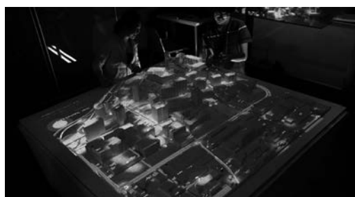
GIS data is used to create “Lego®-tized,” 3-dimensional representations of existing urban areas. The model is augmented with layers of information via projection mapping. Layers: Left: solar insolation; Right: Twitter user activity Photo from MIT Media Lab ( https://www.media.mit.edu/people/jiw/overview/ )
