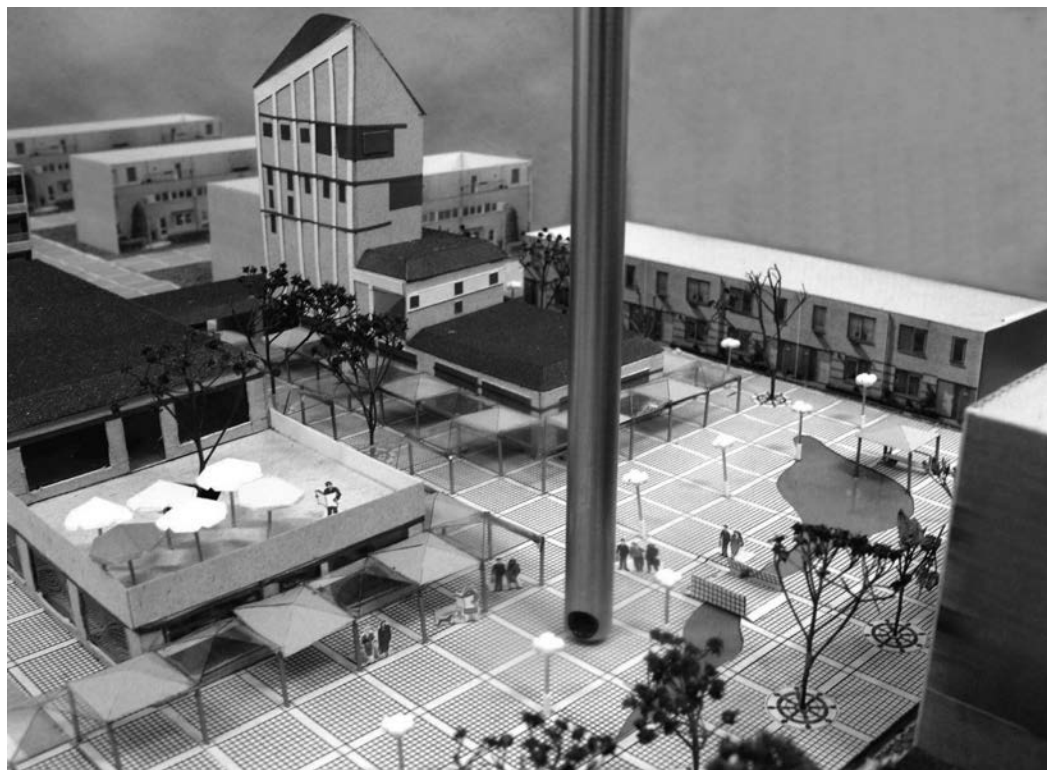
Opto-electronic simulation device with graphic output on a PC monitor or data projector; Recording of the testing of urban atmosphere in the (professional) design model of Bratislava Podhradie location; Endoscope interaction in model, scale M 1:200.
