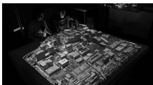
GIS data is used to create “Lego®-tized,” 3-dimensional representations of existing urban areas. The model is augmented with layers of information via projection mapping. Layers: Left: mobility system; Right: Google satellite image Photo from MIT Media Lab ( https://www.media.mit.edu/people/jiw/overview/ )
