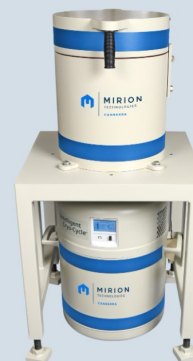
Optimized internal cavity designed for small-sample gamma spectroscopy
