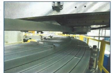
The final turns of the first central solenoid module on the winding table.
