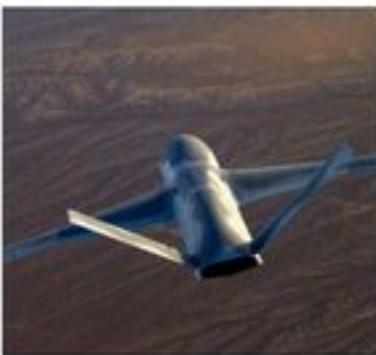
in disaster recovery efforts. NASA uses its Predator B with a sophisticated infrared sensor on its wing to map the intensity and movement of large fires, sharing the information to ensure best use of firefighting resources and streaming video to firefighters on the ground for expanded situational awareness and increased safety.
