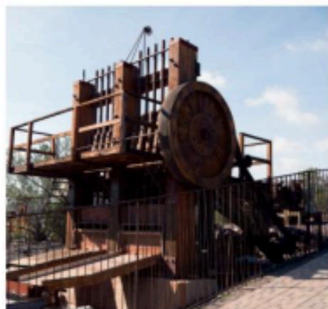
The ten-stamp mill sits outside Cave Creek Museum. (Photo by Pablo Robles)
