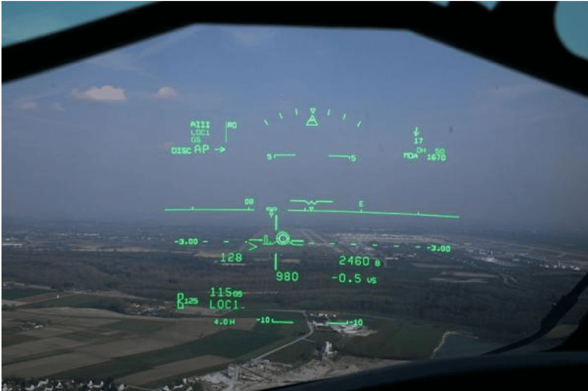
Figure 2.2.3 An example of a HUD in a Bombardier CRJ-200 aircraft at 1000 ft. (Radiant Vision Systems 2021)
