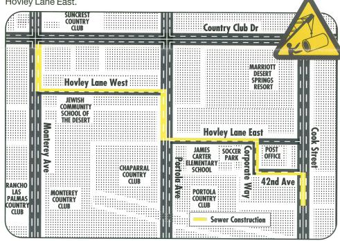
A larger-capacity pipeline is needed to supplement the existing pipeline, which is unsuitable to accommodate the rapid development and future growth for the cities of Palm Desert, Rancho Mirage and portions of Cathedral City. Moreover, the new sewer line will prevent potential sewer spills during peak wet-weather periods when existing trunk sewers are vulnerable.
