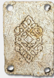
Laser cutting and engraving mycelium
