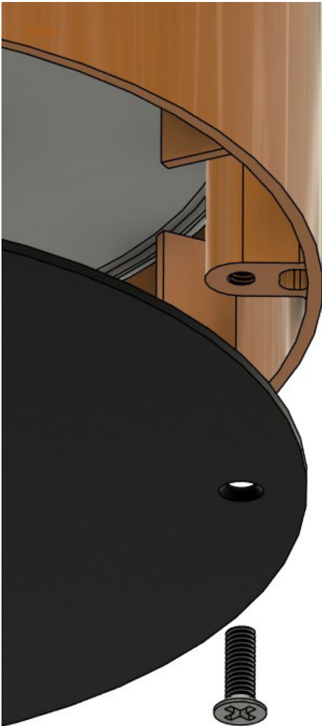
Picture 9: Exterior Assembly Requires Only A Screwdriver
