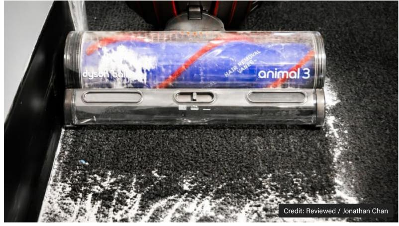
Our testing shows near lossless suction from one edge of the brush head to the other.
