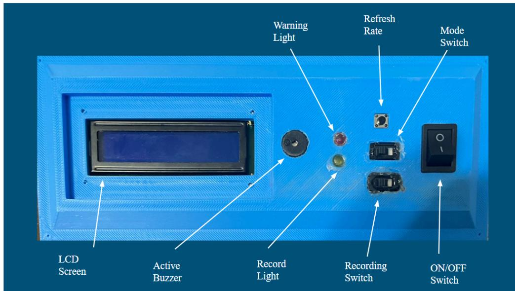
Image 3: Visual to identify all visible switches, LEDs, buttons, buzzers, and screens.
