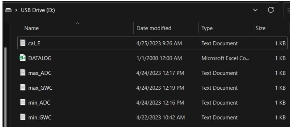
Image 4. Micro SD card files for viewing recorded data or adjusting calibration data.
