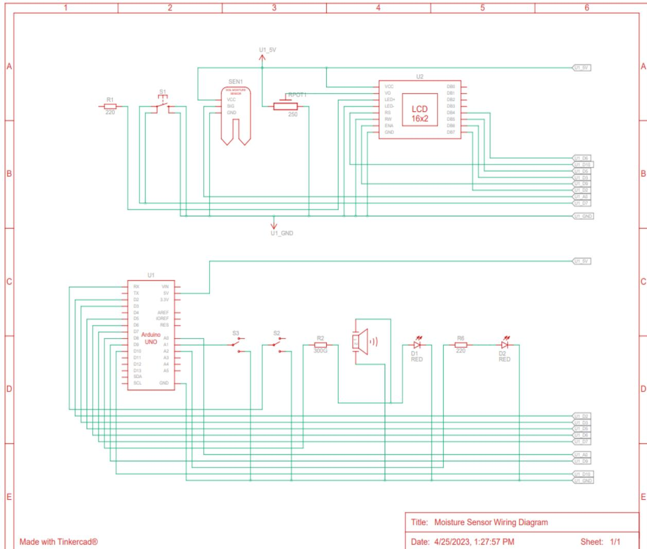
Schematic 1. Wiring diagram for the moisture sensor. This does not include the micro SD adapter.
