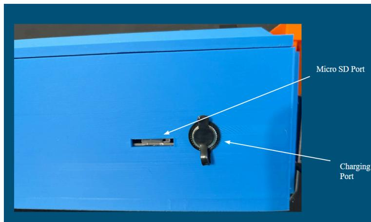
Image 5: Visual to identify the charging port and the micro SD module for data logging.
