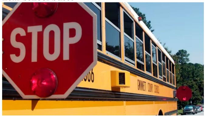
Camera lenses on a Gwinnett County school bus are triggered into recording passing drivers when the bus is stopped.
