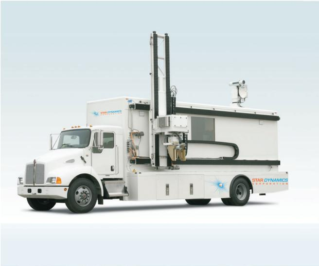
The AMRIS multi-capability, precision-instrumentation radar is an advanced, cost-effective, mobile solution for RCS programs that develop, test, and evaluate stationary targets or dynamic (sea/ground) targets.
