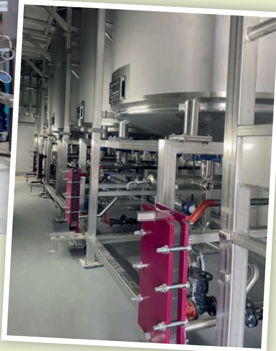
Above: A two-channel CIP system fully integrated into the current system consisting of one 6,000 litre stainless steel water storage vessel, one 10,000 litre stainless steel rinse recovery vessel and one 6,000 litre stainless-steel detergent storage vessel
