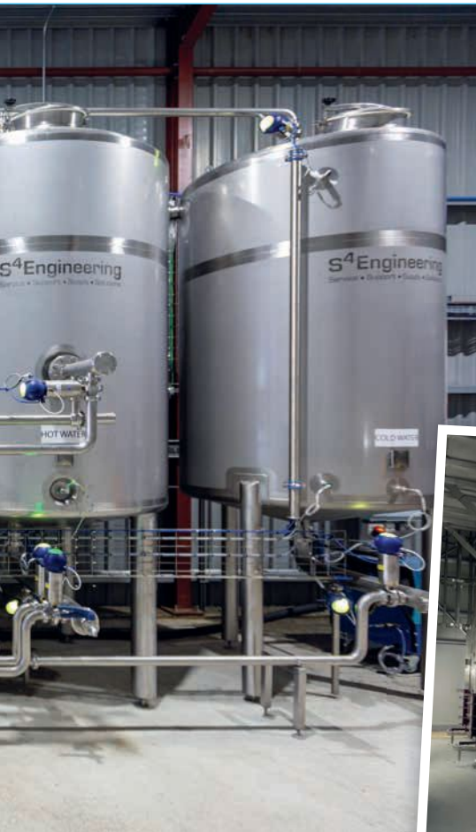
Left: A single-channel CIP set consisting of consisting of one 3,000 litre stainless steel water storage vessel, one 3,000 litre stainless steel rinse recovery vessel and one 3,000 litre stainless-steel detergent storage vessel. The CIP system is a stand-alone plant that is fully automatic and solely operates through a PLC/SCADA control system
