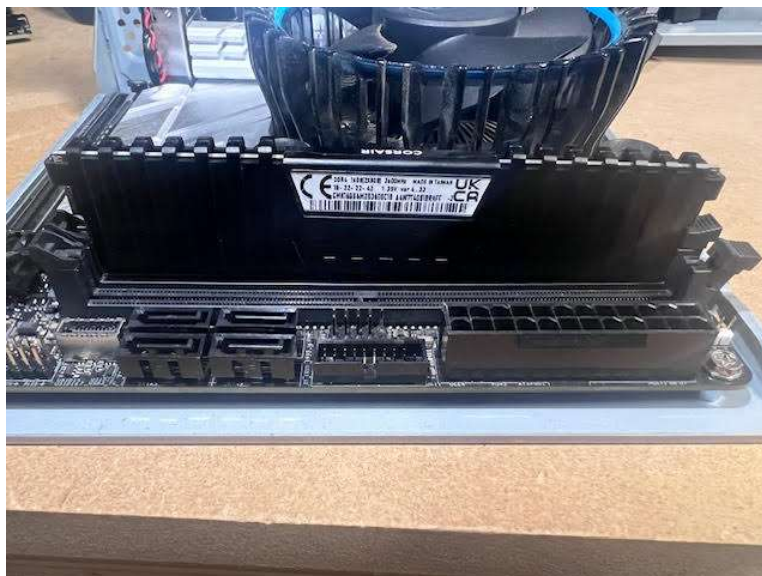
Figure 6: RAM Stick in Position
