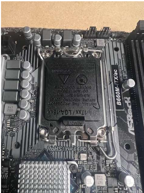
Figure 1: CPU Socket with Plastic Cover
