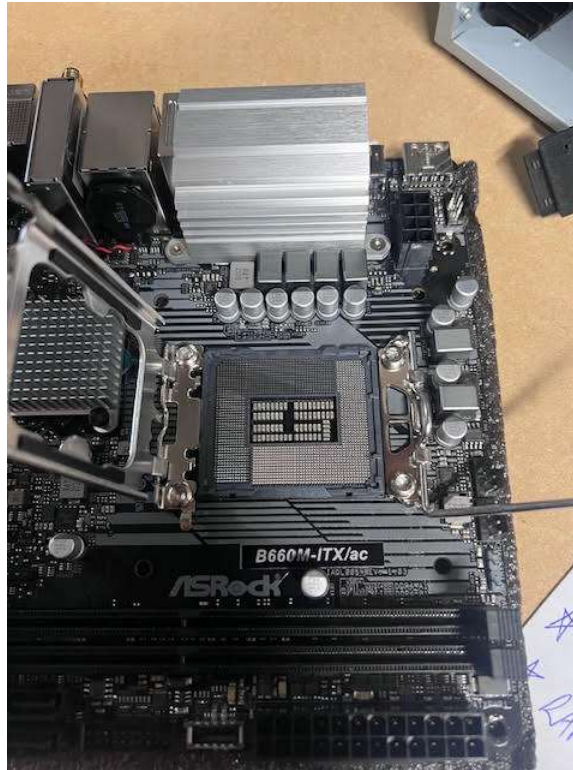
Figure 3: CPU Socket in Open Position
