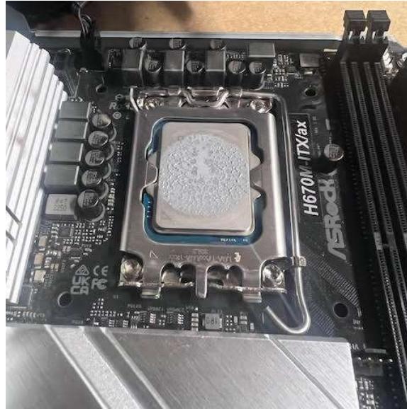
Figure 4: CPU in Position, Showing Thermal Paste from First Contact with Fan
