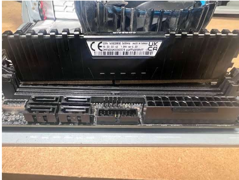
Figure 5: RAM Stick Showing Gap for Socket Divider
