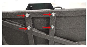
5. Install tire and hand start (3) lug nuts. Torque lug nuts after spare tire is flush with spare tire bracket.
