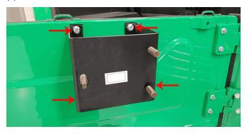
4. Install (4) M8 flat washers, (4) M8 lock washers, and (4) M8 hex nuts on opposite side. Torque nuts to specification.
