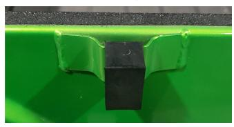
3. Install spare tire mounting bracket with (4) M8 hex bolts and (4) M8 flat washers on bolt head side
