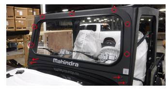
3. Drill (3) 8 mm holes thru each closeout panel at dimple locations on "B" side of panels.
