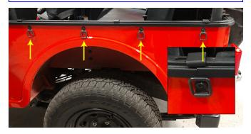
5. Install belt rail "C" clamps over each junction of the side window channel bracket with (8) M6 cap screws (4 per side).
