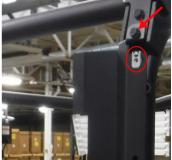
4. Install LH door striker bracket (in wire door hardware kit) to closeout panel bracket. Use (2) M8 nyloc nuts supplied to back of (2) M8 bolts installed in previous step. Repeat on opposite side.
