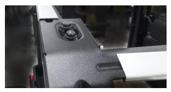
4. Install RH bow bracket to RH ROPS "B" pillar with existing M8 bolts, slide RH bow over bracket.
