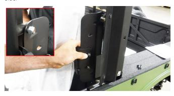
5. Install striker pin and torque to specifications. Repeat on opposite side.
