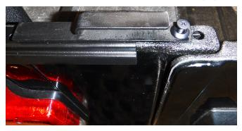
4. Install LH side window channel bracket over belt rail corner brackets. Repeat on opposite side.
