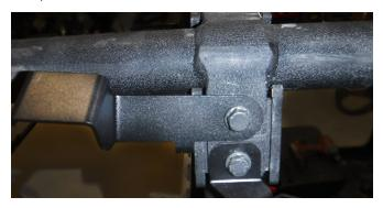
5. Install the RH corner on rear ROPS ("C" pillar) re-using existing M8 bolts from ROPS, then install rear and RH side bow onto RH corner. Secure corner to ROPS with existing bolts.
