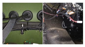
Connect fused red wire from vehicle control harness to keyed power.
