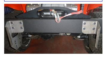
14. Install Mount Beam using (8) 1/2" x 1-1/2" hex head bolts and (8) 1/2" locknuts and hand tighten.
