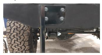
5. Loosely secure driver-side Thrust Plate to Front Plate using (4) 1/2" x 1-1/2" hex head bolts and (4) 1/2" locknuts supplied.
