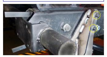
12. Bend both driver's side handles over as shown, then bend passenger side to allow front bumper installation.
