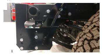
6. Repeat previous step on the opposite side to secure the passenger side Thrust Plate.
