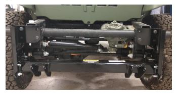
15. Bolts must be installed with heads positioned inside of Mount Beam and locknuts on the outside as shown. This allows clearance for plow spring shackle travel.
