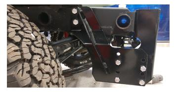
7. Ensure fasteners are tight enough to pull Thrust Plates against vehicle frame. Then use the Thrust Plate as a drill guide to drill (2) 1/2" holes through frame.
