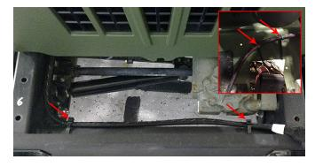
18. Connect vehicle control harness and vehicle battery cable at the four pin connectors.
