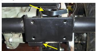
13. Re-install the front bumper with Front Plates using (8) bumper bolts and (8) washers retained from earlier in this procedure, hand tighten only.
