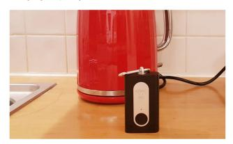
To set up your Atmotube, you charge it for two hours using the cable provided. You'll know when it's fully charged because the LED light will change its colour from orange to green.
