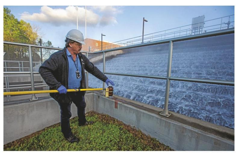
Compliance specialist Bill Burdick caps a sample of effluent water — water that has been treated and is leaving the plant — from the cascades at the T.Z. Osborne Water Reclamation Facility in Greensboro on Tuesday. The water will be tested for 1,4-dioxane at two different independent laboratories.
