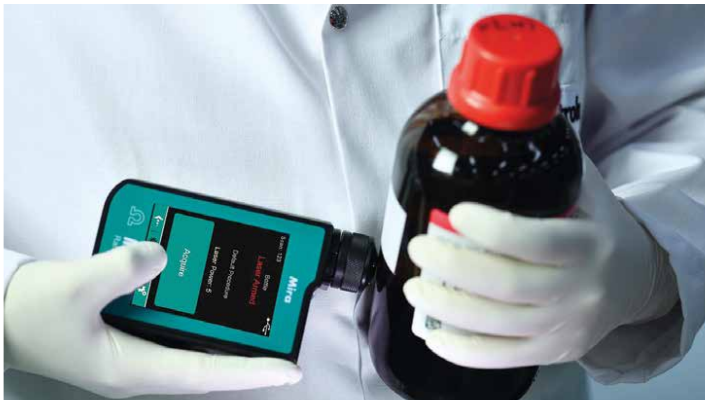
Figure 1. A handheld Raman instrument called the MIRA (from Metrohm) can perform edible oil identification. Source: Metrohm
