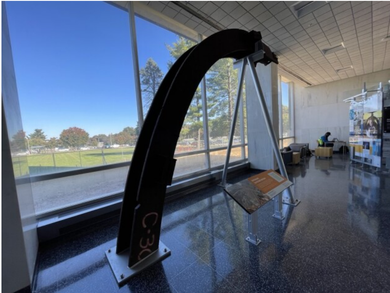
A once-straight steel support column recovered from World Trade Center Tower 2, studied by NIST scientists, on display at NIST headquarters in Gaithersburg, Md.
